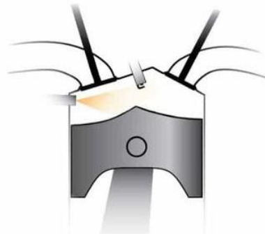
Figure 1: Comparative Illustration of Port Injection and Direct Injection Systems in an Internal Combustion Engine. [Source]
