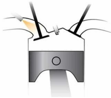
Figure 1: Comparative Illustration of Port Injection and Direct Injection Systems in an Internal Combustion Engine. [Source]
